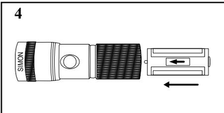
Make sure you place the battery cage in the Flashlight correctly with the 2 positive connections on the batteries pointing towards the front of the flashlight. There should also be a white sticker with RED arrow on the Battery cage, Point that arrow towards the front of the flashlight.
