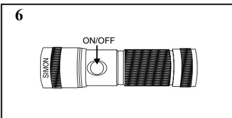
Turn the flashlight On/Off by Pressing the Switch ALL THE WAY DOWN. Then go into a room that you feel has pet urine stains and turn off the lights. The UV Blacklight works best in black out conditions. Point the UV flashlight at the infected areas and you will see discoloration under the UV Blacklight Flashlight.
