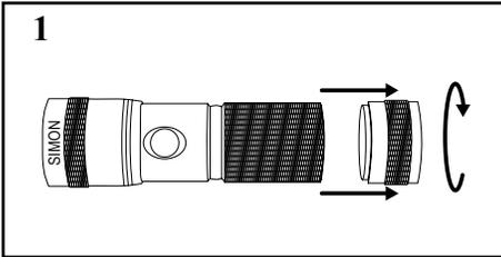
Insert 3 AAA Batteries by unscrewing the rear end Cap and removing the battery cage. Make sure that when you place the 3 AAA Batteries that they are **FULLY CHARGED**.
